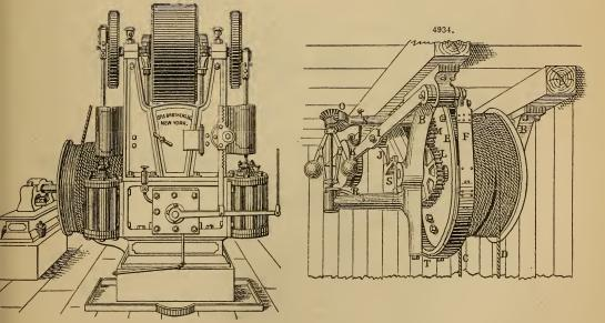
and thence down the shaft. This spool, 4 ft. in diameter, is fixed on an iron shaft c, having at one end a pulley d, of somewhat larger diameter, and at the other end a brake-rim c. Motion is communicated to the pulley d by means of a driving pulley directly beneath it, and an 7 c 2
